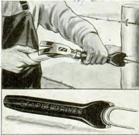
Grooved end prevents driver slipping from staple
